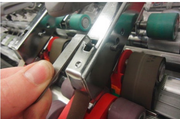
Fig. 12: Wrong position of Elispring – check gauge too high
