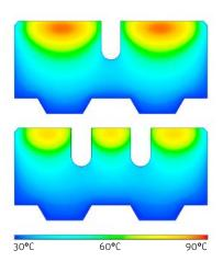
Fig. 1: SUESSEN TwinDisc, new standard: comparison of heating characteristics of tires with 1 or 2 cooling grooves respectively at identical rotor speed
