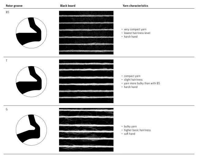
Influence of rotor groove on yarn characteristic, example 100% viscose Ne 20
