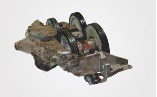
Comparison of bearing with ProFiL Cartridge (left) with oil-lubricated bearing (right) after 8 weeks of application spinning 100 % cotton, Ne 24 at 120 000 rpm on the same machine
