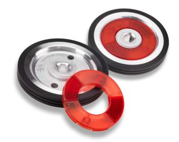
The power consumption of TwinDisc bearings is not influenced by the shape of the revolving components, but considerably by the TwinDisc tires. In contrast with the discs of other manufacturers, the energy consumption of SUESSEN TwinDiscs is lower (see Fig. 3). Hence at a rotor speed of 120 000 rpm about 4.0 W per spinning position is saved compared to the competitors' discs.
