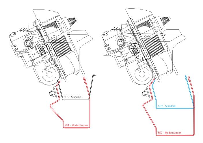
In fact, the only component to be replaced is the trash channel. The complete drive system of the trash conveyor belts is reused as well as the conveyor belts themselves. Consequently maintenance, settings and spare parts of the trash removal system remain the same. This is very comfortable for your spare parts stock and the maintenance personnel.
